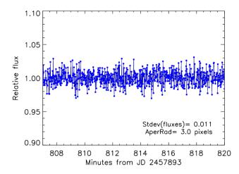
**Figure 9.** The negative light curve obtained from the 1.23-m telescope at Calar Alto Observatory (Almería, Spain). This is the best light curve, in terms of flux dispersion, closest to the shadow limb of  $2002 \text{ GZ}_{32}$ . Calar Alto is located at a projected distance on the sky plane of 307 km south from the centre of the limb fit, following the ellipse major axis direction (i.e. the direction of the major axis of an equatorial ring).
