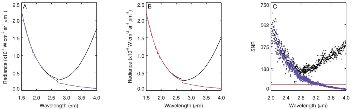
**Fig. S2. Thermal tail removal and resulting signal-to-noise ratio.** (A) A typical Benu radiance spectrum, with and without thermal tail removal (blue and black curves, respectively). (B) A redder Benu radiance spectrum, with and without thermal tail removal (red and black curves, respectively). (C) SNR at the pixel level (before resampling), for a typical Benu spectrum with and without thermal tail removal (blue and black, respectively). SNR=50 is indicated by the line.
