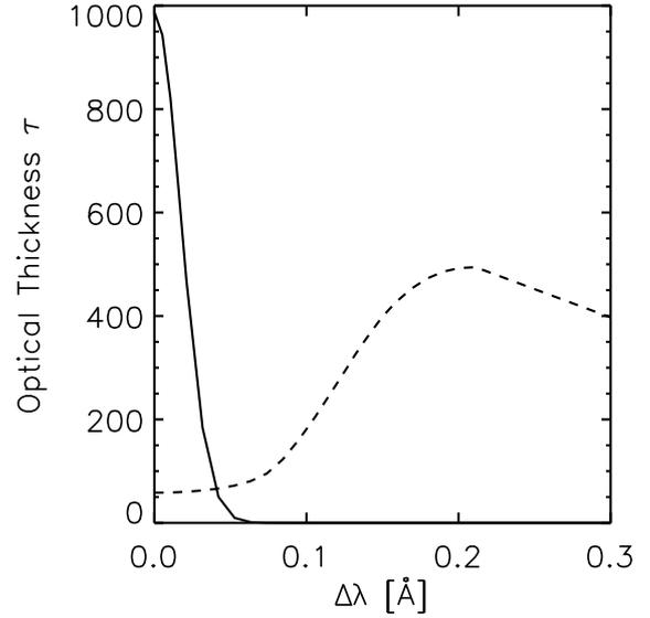
**Fig. 11.** Theoretical optical thickness  $\tau$  of fibril within Mg II h line (solid line) calculated with 2D codes using our fibril model, and the theoretical Mg II h line profile for the CB C modified model 65-4 (dashed line) calculated using our NLTE chromospheric codes. The fibril model parameters are  $D = 2000$  km,  $T = 10\,000$  K (isothermal),  $p = 2$  dyn cm $^{-2}$  (isobaric). The  $x$  scale is given in Å (0.1 Å corresponds to 4.5 km s $^{-1}$ ).
