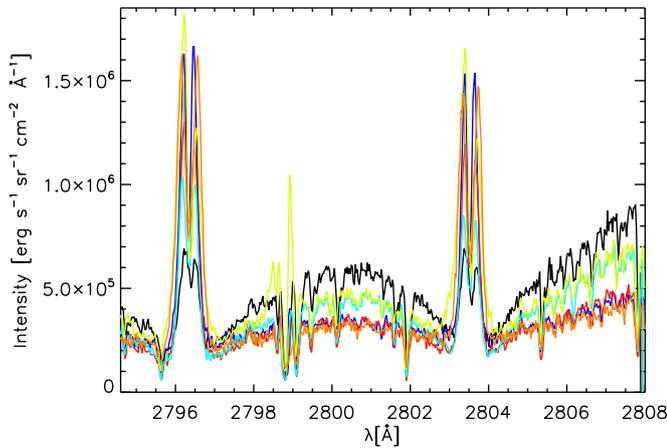
**Fig. 7.** Intensity profiles of Mg II lines for events that have high intensity in the wings and small intensity in the peaks. The selection was done randomly (see the small circles in Fig. 3). The correspondence is as follows: 5 – dark blue; 6 – light blue; 7 – red; 8 – orange; 9 – light green. The black line represents the E profile. All these profiles have a shape between CB C and CB E profiles.
