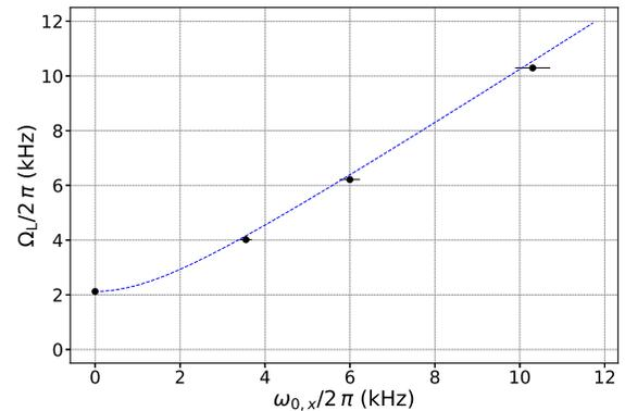
FIG. 4.  $\Omega_L$  vs  $\omega_{0x}$  as a test of the spin anisotropy, for an applied  $p = 1$  tuning field,  $\Omega_t/2\pi = 0.354(3)$  kHz, and other parameters as in Fig. 1. Blue dots for data and continuous line for the theoretical predictions. Error bars two per thousand on the frequency, and 4% on the  $\omega_{0x}$  scale.
