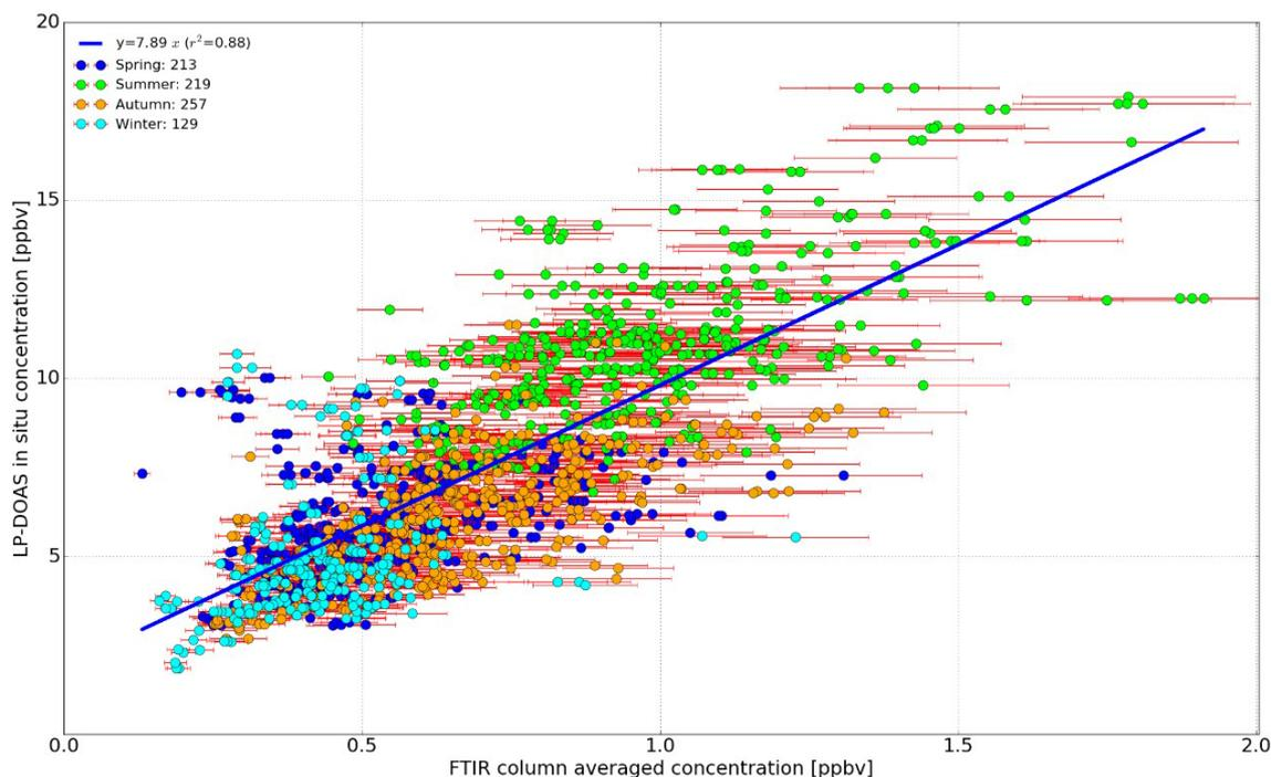
**Figure 3.** Correlation plots of FTIR  $X_{\text{HCHO}}$  measurements against LP-DOAS ground-level HCHO measurements. The blue lines are linear-fitted curves of respective scatter points. All concurrent data pairs were grouped by season. The number of data pairs within each season was also included.
