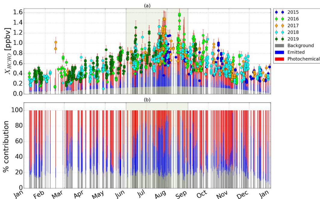
**Figure 5.** (a) Separation between emitted and photochemical HCHO by using CO–O<sub>x</sub> tracers to model FTIR observations. (b) Relative contributions of emitted, photochemical and background sources to the observed  $X_{\text{HCHO}}$  from 2015 to 2019 over Hefei, eastern China. The grey vertical shaded area indicates summertime measurements.
