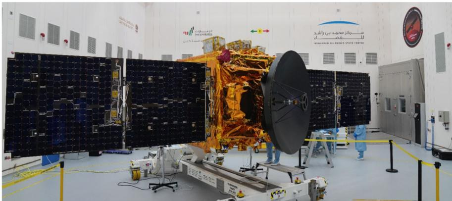
**Fig. 21** EMM observatory solar array deployment testing
