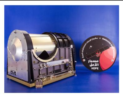
Fig. 4 The EMIRS flight instrument
