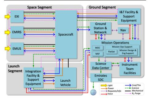
Fig. 9 Block diagram showing the relationship between the launch, space, and ground segments of EMM
