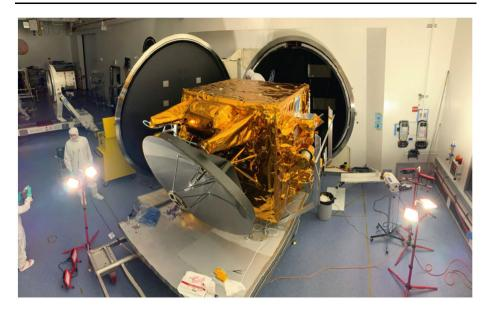
Fig. 20 Preparation of the EMM observatory for thermal vacuum testing
