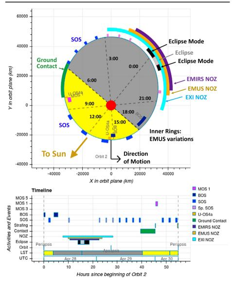
**Fig. 7** Diagram of an "orbit in the life" of EMM, with sample color-coded observation sequences, NOZ locations, and ground contact indicated as viewed from above Mars (top) and on an orbit timeline (bottom). The orbit start and stop location is at midnight LST, and yellow and gray shading indicate the sunlight and shadowed parts of Mars
