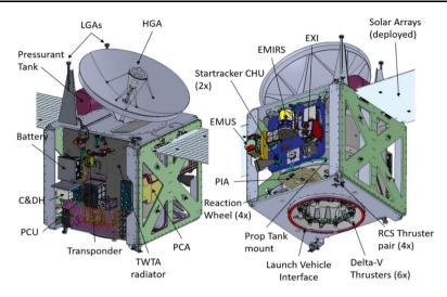
Fig. 15 CAD drawing of EMM spacecraft showing the locations of important components, including the science instruments EXI, EMIRS, and EMUS
