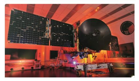
Fig. 13 EMM Hope Probe undergoing solar array testing
