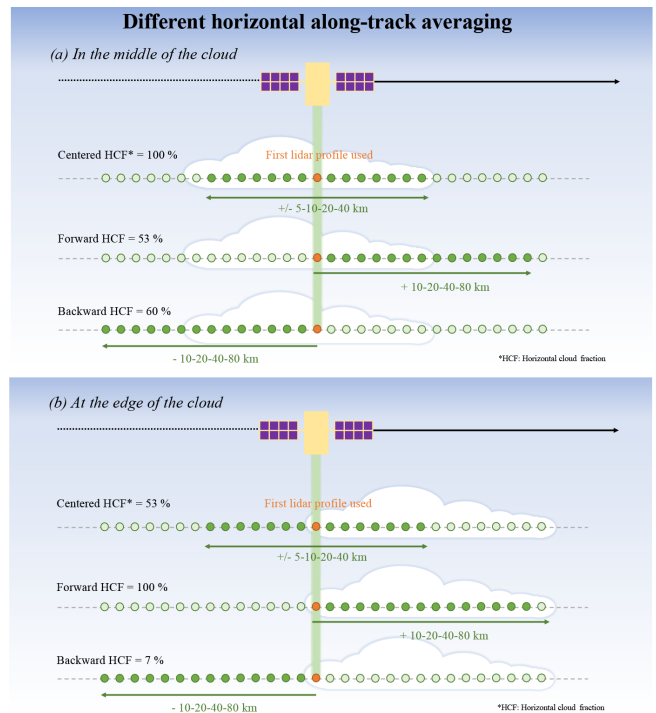
Figure 3. Illustration of the horizontal along-track averaging that is used by the DA to compute the horizontal cloud fraction (HCF): (a) the lidar beam is in the middle of the cloud and (b) the lidar beam is at the edge of the cloud. The dark-green circles correspond to the profiles used in the different horizontal averaging scenarios (centered, forward or backward).
