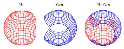
Figure 5. The Yin–Yang grid is a combination of two limited-domain latitude–longitude grids assembled to provide complete coverage of the sphere.
