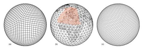
Figure 1. (a) A cubed-sphere grid. (b) An icosahedral (triangular) grid with additional refinement over Europe, as indicated in red. (c) An icosahedral (hexagonal) grid.
