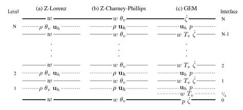
**Figure 7.** (a) A Lorenz-type variable staggering for a model utilizing height coordinates, (b) a Charney–Phillips-type variable staggering for a model utilizing height coordinates, and (c) a modified Charney–Phillips-type staggering used in the GEM model that introduces a new near-surface level for vertical velocity and temperature.
