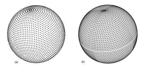
**Figure 4.** Locations of the octahedral reduced Gaussian grid nodes (**a**), and the edges of the primary mesh connecting the nodes as applied with the finite-volume discretisation in FVM (**b**). A coarse octahedral grid with only 24 latitudes between each pole and the Equator ("O24") is used for illustration. The dual mesh resolution of the octahedral reduced Gaussian grid is about a factor of 2 finer at the poles than at the Equator; see Smolarkiewicz et al. (2016).
