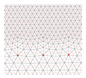
**Figure 2.** Detail of one step of local mesh refinement used by the OLAM Voronoi mesh. The transition zone is constructed by explicit topological reconnection of the grid lines, which produces pairings of heptagons (red dots) and pentagons (blue dots) along the refinement perimeter.
