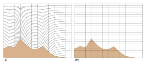
Figure 8. (a) A terrain-following coordinate passing over rough topography. (b) A cut-cell coordinate used for representing the same topography.
