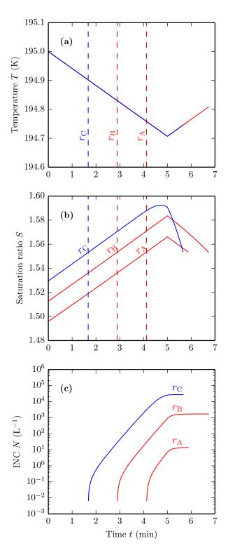
**Figure 10.** Evolution of temperature (a), saturation ratio (b), and INC (c) for three air parcels with slightly different initial water vapour mixing ratios:  $\{r_A = 1.78; r_B = 1.80; r_C = 1.82\} \times 10^{-5} \,\mathrm{kg \, kg^{-1}}$ . The parcels follow the same temperature time series as shown in (a), but they begin nucleation at different times (indicated by the dash lines) and end up with widely different INCs.
