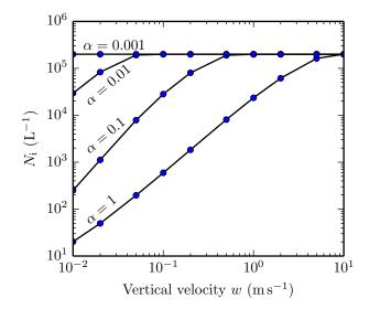
**Figure 2.** INC obtained from homogeneous nucleation at 195 K forced by constant vertical velocity w for different values of the deposition coefficient  $\alpha$ .
