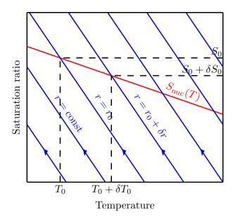
**Figure 3.** Diagram illustrating the initial conditions of the air parcels. Prior to nucleation air parcels follow isolines of water vapour mixing ratio r (shown here in blue) and approach the curve  $S_{\text{nuc}}(T)$  from below (as indicated by the arrows). Nucleation begins at the intersections of the r isolines with the curve  $S_{\text{nuc}}(T)$ .
