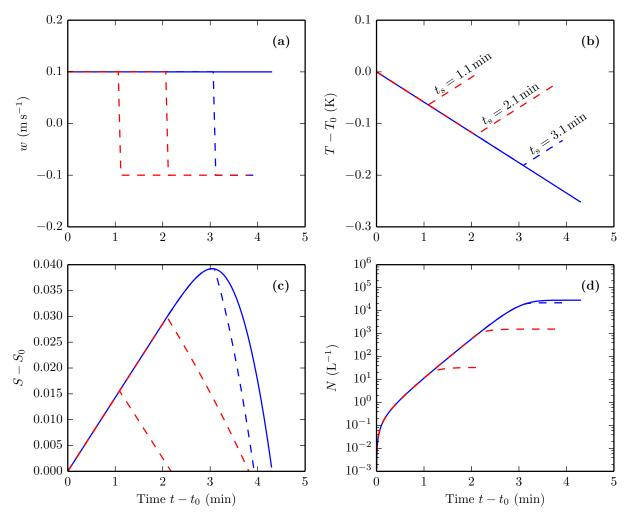
**Figure 5.** Evolution of vertical velocity (a), temperature (b), saturation ratio (c), and INC (d) during nucleation events forced by constant  $w = 0.1 \,\mathrm{m\,s^{-1}}$  (solid) and by  $w = \pm 0.1 \,\mathrm{m\,s^{-1}}$  (dash) as defined by Eq. (7). Blue curves show vapour-limit events and red curves show temperature-limit events.
