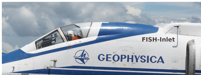
Figure 5. Side-mounted FISH inlet at Geophysica (photo: Armin Afchine).
