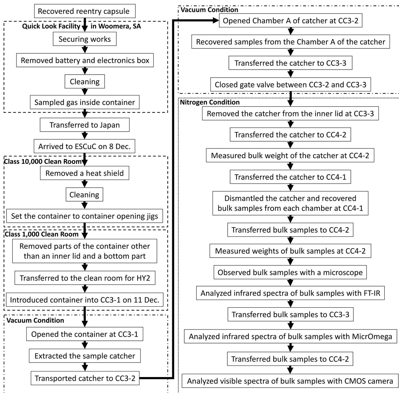
**Extended Data Fig. 1 | A flowchart of a series of processes for the Hayabusa2 sample container and its catcher experienced after its landing.** A flowchart of a series of processes for the Hayabusa2 sample container and its catcher experienced after its landing. Note that samples inside the container were only exposed to vacuum and nitrogen environment in the clean chambers for Hayabusa2-returned samples.
