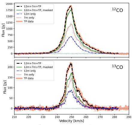
**Figure 1.** Integrated flux spectra for the CO(2–1) (top) and <sup>13</sup>CO(2–1) (bottom) cubes at 0.25 kms<sup>-1</sup> resolution. The cubes compared are the feathered cube (*black dashed line*), the total power array data only (*thick pink line*), the 7 m array data only (*red dotted line*), and the 12 m array data only (*blue dotted-dashed line*). A solid green line shows the flux in the feathered cubes after applying the dilated mask described in Section 3.1.
