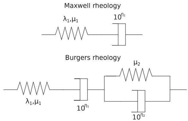
**Figure 1.** Mechanical diagram of Maxwell and Burgers rheologies.
