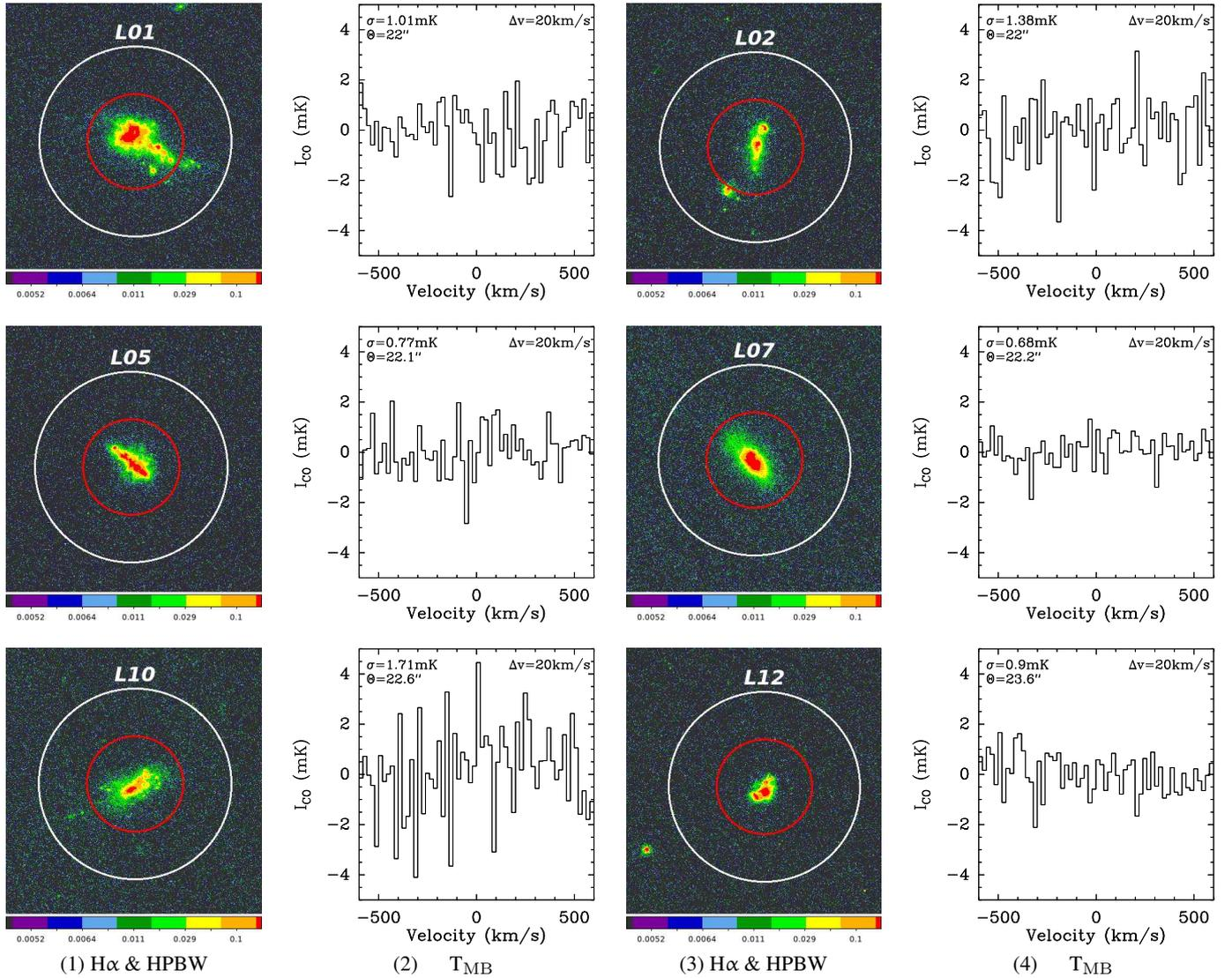
**Fig. 2.** CO(1–0) non-detections of LARS galaxies. The beam size for the CO(1–0) transition is shown in *Cols. (1) and (3)* as white circle on top of our HST H $\alpha$  narrow band images. The measured signals on the main beam brightness temperature scales are shown in *Cols. (2) and (4)*.
