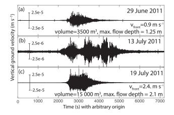
**Figure 4.** Seismograms of three debris flows recorded at station IGB02. The event on 19 July 2011 (c) is analyzed in the present study. Burtin et al. (2013) focused on the event on 13 July 2011 (b). Note the different *y* scales. Debris-flow parameters in (a) and (c) are calculated following Schlunegger et al. (2009) using unpublished data by the Swiss Federal Institute for Forest, Snow and Landscape Research WSL. All shown time series were filtered between 0.5 and 5 Hz.
