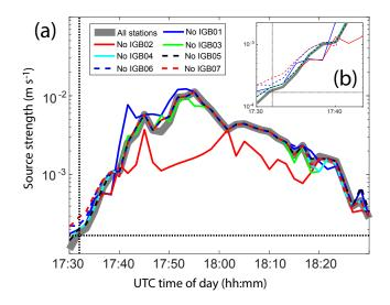
**Figure 11.** (a) Variations in calculated source strength  $A_0$  as individual stations are removed. Vertical and horizontal bars indicate earliest detection time at 17:32 UTC and proposed threshold, respectively. (b) Magnification of near-earliest detection time at 17:32 UTC.
