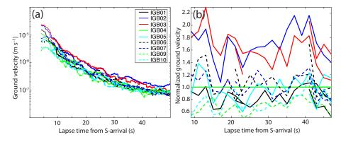
Figure 12. Coda amplification analysis. (a) S-wave coda envelopes of an M2.2 earthquake on 15 July 2011 (epicentral distance: 12 km). Bold lines indicate lapse times greater than twice the S arrival time. (b) Coda amplification with respect to station IGB04 using signals of the three earthquakes listed in Table 3.
