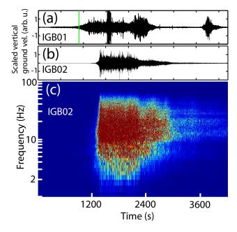
**Figure 5.** Debris-flow seismograms at stations IGB01 and IGB02 (**a**, **b**) and spectrogram of station IGB02 (**c**). Green bar in (**a**) denotes 17:35 on 19 July 2011. Note the second seismic burst after 3600 s likely represents a local mass motion event near IGB01. For illustration purposes, a bandpass filter between 0.01 and 50 Hz has been applied to the time series (IGB01 and IGB02 are flat between 1 and 100 Hz and between 0.033 and 50 Hz, respectively, as specified in Table 1).
