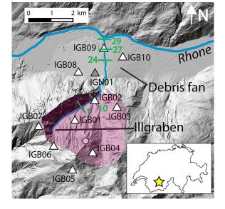
**Figure 1.** Illgraben region with its upper-catchment area (shaded polygon) and debris fan in the Rhône Valley. Numbered green lines represent check dams 1, 10, 24, 27 and 29; 2011 seismometer locations are indicated by triangles (grey triangle represents the 2015 noise record station) and a WSL rain gauge is indicated by the circle. The inset shows outlines of Switzerland and the yellow star marks the location of Illgraben.
