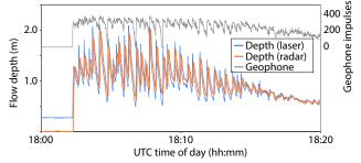
Figure 3. Flow depth and geophone impulses of Illgraben debrisflow event on 19 July 2011 (recorded near check dam 29).
