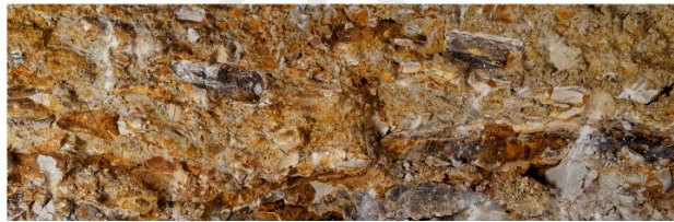
b) Incoherent and marly limestone (depth=10 m)
