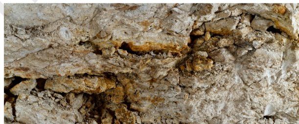
c) Fractured limestone rock (depth=16 m)
