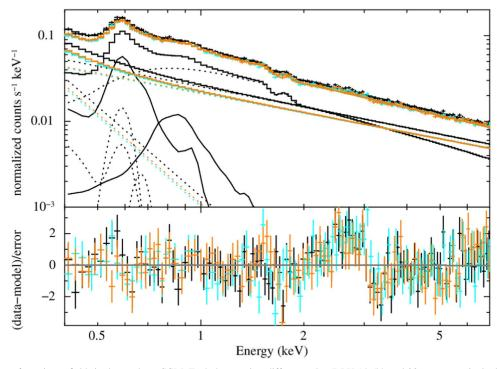
**Figure 7.** Stacked spectra of consistent fields in the northern CGM. Each detector is a different color (DPU 14, 54, and 38 are, respectively, black, orange, and cyan). The model for the CGM is two APECs, marked in solid black lines. Background and foreground components are marked in dashed lines. Model components that are identical between each detector are only shown once. The feature around 3 keV is due to the data filtering procedure as described in the text.
