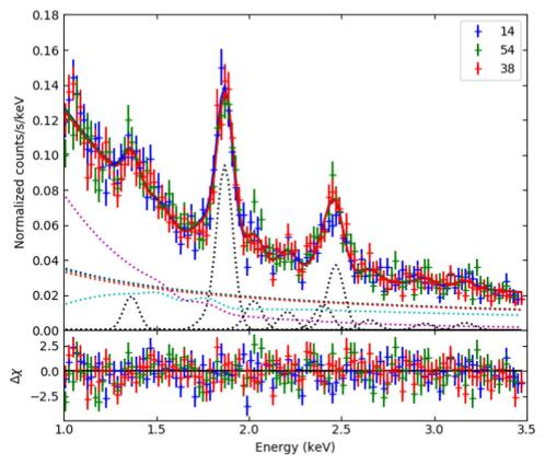
**Figure 11.** X-ray spectra of Cas A. Data are shown for all three DPUs: 14 = red, 54 = green, and 38 = red. The fitted instrumental background for each DPU is shown as a dotted curve with the same color as the data. The dotted cyan curve is the cosmic X-ray background. The dotted magenta curve is the power law from Cas A. The dotted black curves are the Gaussian emission lines.
