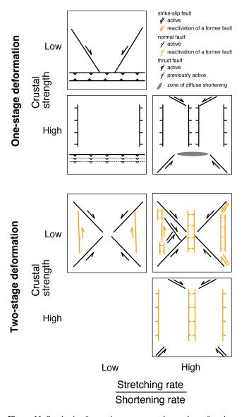
**Figure 11.** Synthesis of map view structures observed as a function of crustal strength, ratio of stretching/shortening rates, and tectonic inheritance. For the two-stage deformation, newly formed faults are in black and reactivated faults are in orange.
