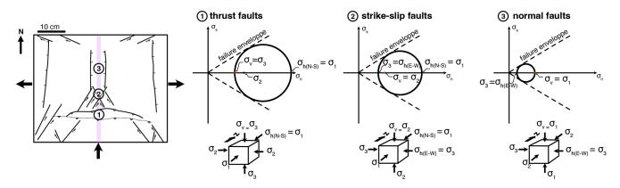
Figure 8. Interpreted distribution of structures for model BI05 after 7.7% of shortening and corresponding principal stress axis and Mohr–Coulomb analysis for the areas with labels 1, 2, and 3 on the left figure.
