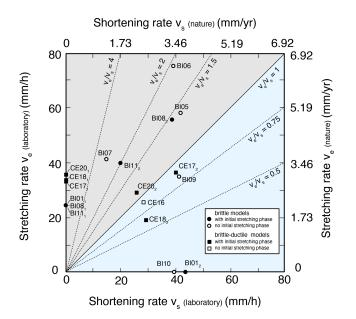
**Figure 3.** Applied boundary kinematic conditions for models with brittle crust (circles) and brittle–ductile crust (squares). Models with two-stage deformation have black filled symbols and subscripts to indicate the stage of deformation. Laboratory and scaled values are given for the shortening and stretching rates.
