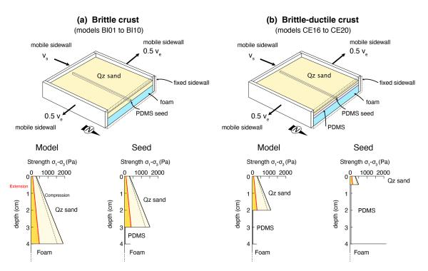
**Figure 2.** Experimental setup (top) and corresponding strength envelopes (bottom) under extension and compression for (**a**) models with brittle crust ("strong" crust) and (**b**) models with a brittle–ductile crust ("weak" crust). Solid lines correspond to the peak friction for Qz sand and dashed lines to the reactivation friction.
