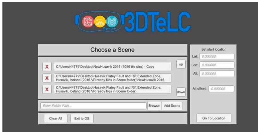
Fig. 5. Screenshot of the selection tool used to choose the scene files for virtual reality viewing in GeaVR. The scene files are created from the Photoscan OBJ output files using the converter and are available to download from http://www.3dtelc.com along with the converter and viewing software.
