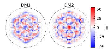
**Fig. 4.** Example of DM commands on both continuous deformable mirrors produced by the SM algorithm that can generate a DH on HiCAT. The DM commands in units of OPD is an approximation of the introduced deflection. The black circle represents the active area of the continuous DMs. For scaling comparison, IrisAO segments are plotted in transparency. The segment footprints are not realistic here as the DM2 is out of the pupil plane.
