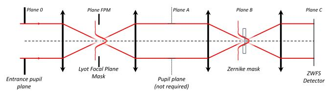
Fig. 1. Schematic diagram of the ZWFS downstream of a binary amplitude FPM. The light in the entrance pupil comes from the telescope and deformable mirrors in plane 0. It is focused on the FPM, which is re-imaged on the Zernike mask in plane B. The intermediate pupil plane A is not required.
