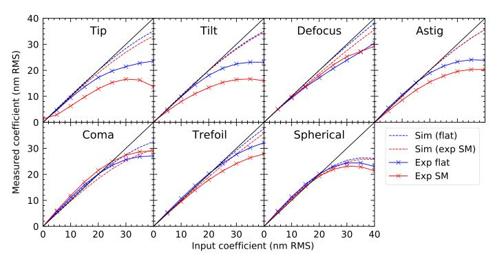
Fig. 5. Response curves of the ZWFS to low-order Zernike modes, in simulation (dotted lines) and from HiCAT experiments (solid lines with cross markers). The ZWFS has been calibrated around the DM flat maps that optimize wavefront quality. Response curves are measured both around these flat maps (blue curves) and around SM commands (red curves).
