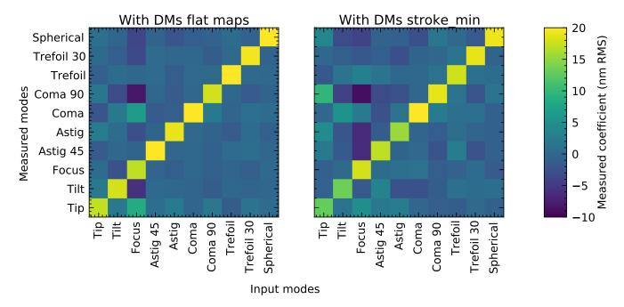
**Fig. 6.** Mode coupling matrix of the ZWFS to Zernike modes using a Jacobian matrix calibrated with Zernike modes around flat DMs. Introduced and measured modes are given on the horizontal and vertical axes. *Left*: with flat DMs. *Right*: after introduction of SM offset on the DMs. Modes are introduced with 20 nm RMS in each case.
