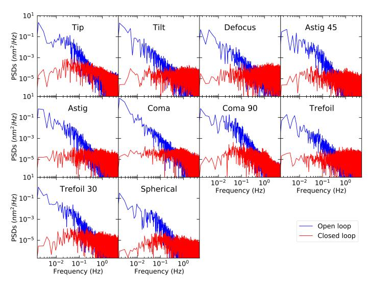
Fig. A.1: Temporal PSDs for ten Zernike modes from tip to spherical aberration, in open-loop (blue) and closed-loop (red) operations. The data are related to the experiment presented in Sect. 4.2.
