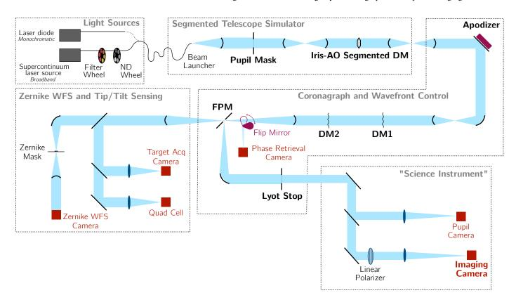
Fig. 3. Semi-unfolded layout of the HiCAT testbed. The apodizer labeled in the *top right* corner of the diagram is currently replaced by a flat mirror.
