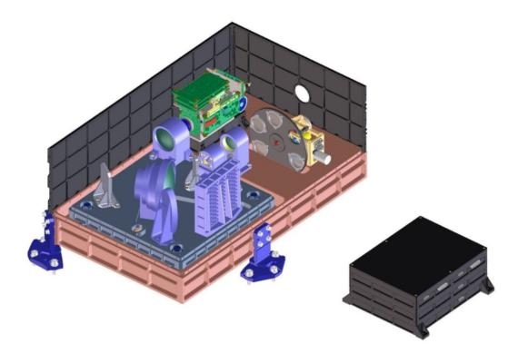
The VenSpec-H instrument is comprised of two boxes as shown above, the instrument box and the electronics box. The instrument box contains a warm base plate (0°C operating temperature) where the filter wheel and detector/cooler are mounted, and a cold base plate (-45°C operating temperature) where the majority of the optical elements are mounted. The majority of the electronics are in a separate box to improve the thermal stability of the instrument box.
