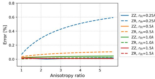
**Figure 12.** Error of the isotropic Rayleigh wave speed estimates due to anisotropic incidence. The isotropic model  $N_k = 0$  (eqs 17 and 18) is used for the non-linear regression. The error is the difference between the target value and estimate, scaled by the target value of  $2 \text{ km s}^{-1}$  (eq. 16). Errors are displayed as a function of the anisotropy ratio explained in Section 2.5. Results are presented for different components and maximum fitting ranges  $r_{fit}$ .
