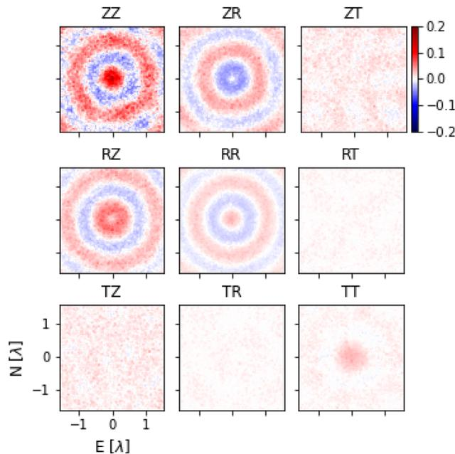
**Figure 16.** Focal spots at 10 Hz in a homogeneous elastic half-space obtained with 10 per cent variance Gaussian noise added to the source-mirror Green's functions  $G$  (eq. 1). The implementation is described in Section 2.6.
