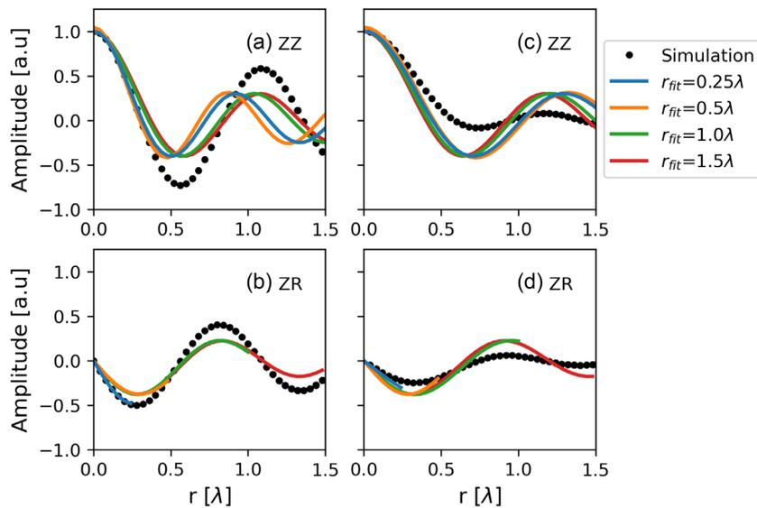
**Figure 13.** Non-linear regression results for anisotropic incidence using the assumption of medium anisotropy  $N_k = 14$  (eqs 18 and 19). Results are shown for estimates over different fitting ranges  $r_{fit}$  for the ZZ and ZR component focal spots. Data from Fig. 10(a) obtained with the anisotropic incidence pattern shown in Fig. 9 are plotted along the north and east axis. (a) ZZ and (b) ZR data along the north axis. (c) ZZ and (d) ZR data along the east axis.
