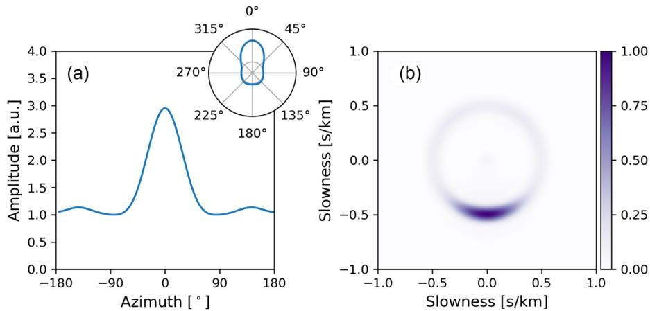
**Figure 9.** Parametrizations of anisotropic surface wave incidence. (a) Azimuthal distribution of the weights  $w_m$  (eq. 13) applied to the seismograms simulated at the mirror elements  $m$ . (b) The corresponding beamforming pattern obtained from ZZ component correlations shows the strong incidence from north.
