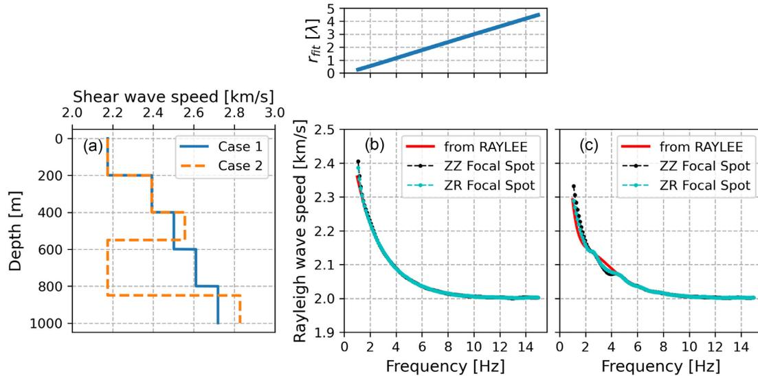
**Figure 15.** Focal spot based dispersion estimates. (a) Depth dependent shear wave distributions of the two layered elastic half-spaces used to simulate dispersion. (b), (c) Dispersion curves obtained from focal spot measurements (black) compared to theoretical fundamental mode dispersion curves (red) obtained with the RAYLEE solution of Haney & Tsai (2017). Data in (b) and (c) correspond to the Case 1 and Case 2 profiles in (a).
