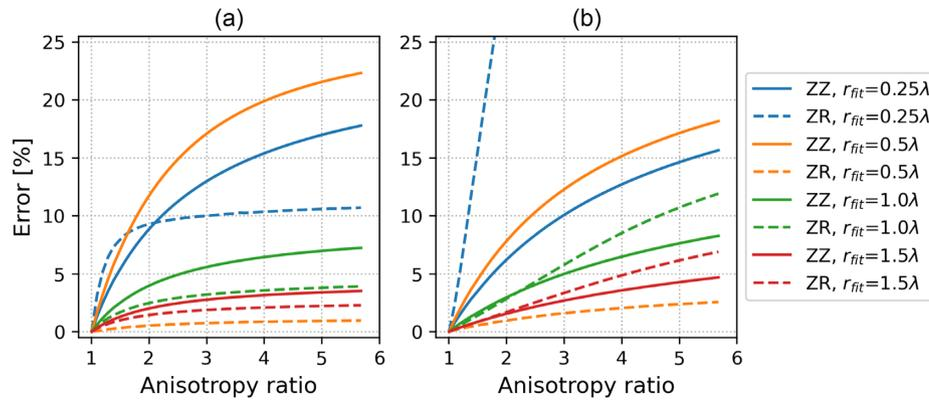
**Figure 14.** Error on Rayleigh wave speed estimates for anisotropic incidence using the assumption of medium anisotropy. Errors are displayed as a function of the anisotropy ratio explained in Section 2.5. Medium anisotropy is assumed in the non-linear regression (eqs 18 and 19, with  $N_k = 14$ ). Results along (a) the north direction and (b) the east direction are presented for different maximum fitting ranges  $r_{\text{fit}}$  and components ZZ and ZR.
