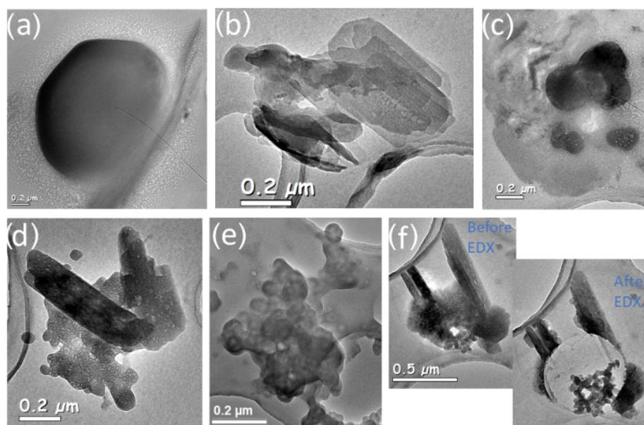
**Figure 6.** Assorted sea salt particles. (a)  $\sim 1.5\ \mu\text{m}$  rounded NaCl, Gold 1; (b)  $\text{CaSO}_4$ , Gold 1; (c) NaCl and Mg, Gold 1; (d)  $\text{Na}_2\text{SO}_4$  with K, Gold 1; (e)  $\text{NaNO}_3$  mixed with BC, Gold 24; and (f) BC encapsulated in  $\text{Na}_2\text{SO}_4$  with K, Gold 1.
