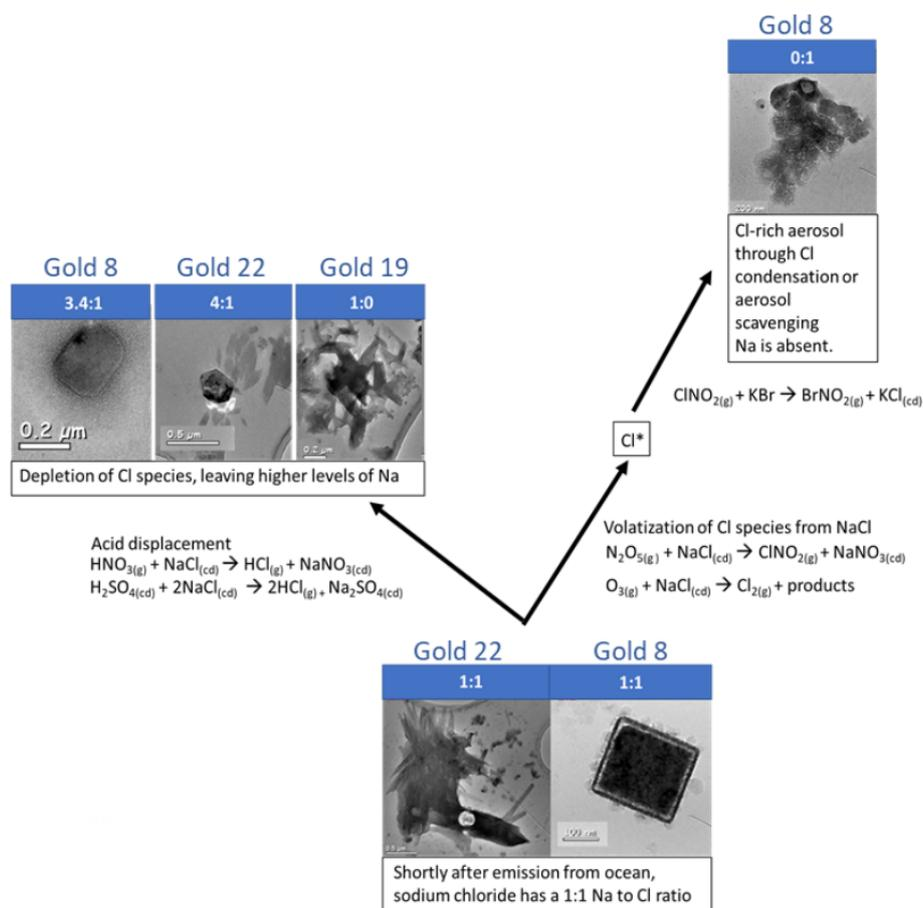
**Figure 5.** Schematic showing different stages of sea salt conversion with example mechanisms. The particles are from CLARIFY filters and range from sea salts which have been freshly emitted to Cl-depleted particles containing nitrates and sulfates. Cl aerosol formation is also shown. Na : Cl ratios showing depletion of Cl with sea salt conversion are shown in the bar above each particle image.
