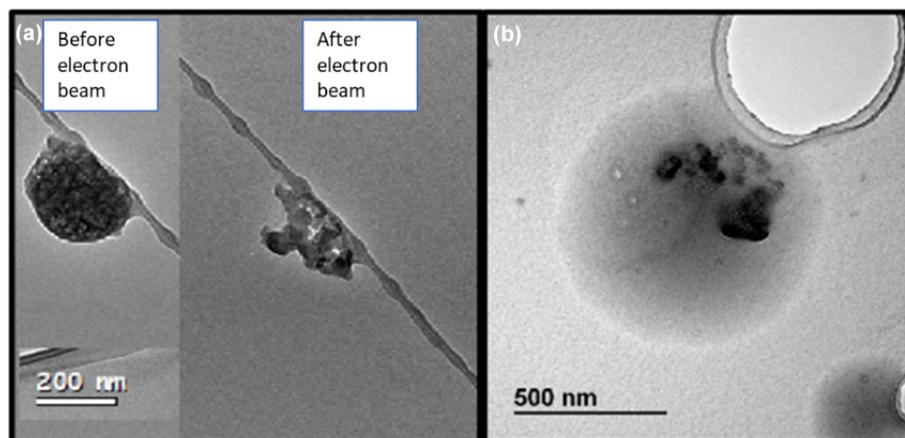
**Figure 4.** Potassium salt in a core–shell morphology around a refractory BC core (a) and organic aerosol with interstitial K salt (b). Note the difference in scale between the two images.
