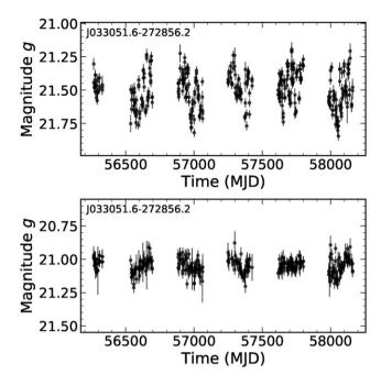
**Figure 3.** Example PSF (top panel) and DIA (bottom panel) light curves of a resolved variable galaxy. The PSF light curve includes additional false variability due to seeing variations. Significant intrinsic variability is still detected in this source using DIA photometry. The slight difference in magnitude for resolved sources is due to the larger area enclosed in the DIA aperture.
