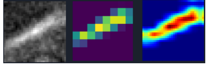
Fig. 9. Illustration the Grad-CAM function that helps identifying the regions of interest in the image that triggered the O'TRAIN classification. Left: residual cutout ( 32 \times 32 pixels) of a bogus identified in the JAST telescope images. Center: the GRAD-CAM Heatmap ( 8 \times 8 pixels) showing the final feature maps \times their importance where our O'TRAIN CNN focused on to take its decision. Right: rescaled Grad-CAM heat map ( 32 \times 32 pixels) for a direct comparison with the cutout.
