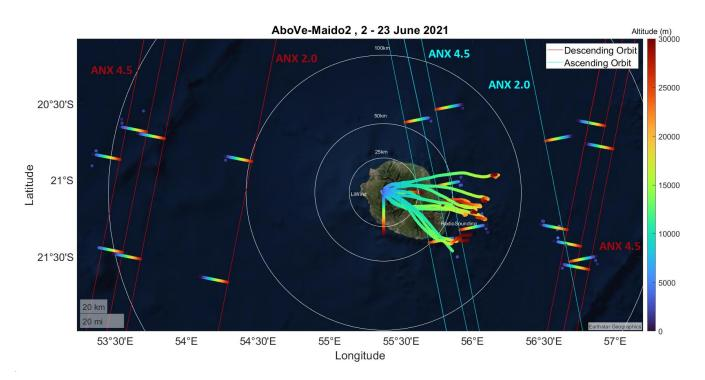
Figure 1. AboVE-Maido 2 Campaign overview with ascending and descending Aeolus overpasses in cyan and red. The colored trajectories represent the ascending phase of the radiosondes, with their altitude shown through a colormap. The ascending node crossing configuration is specified for each Aeolus overpass. Credit: base map sources are Earthstar Geographics.
