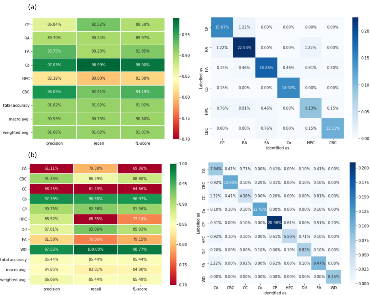
Figure 4. Evaluation of training for each probe with an independent test set. (a) Left, classification report (PIP) obtained for the corresponding test set. Right, confusion matrix (PIP) obtained for the corresponding test set; values on the diagonal correspond to samples correctly classified. (b) Left, classification report (2DS) obtained for the corresponding test set. Right, confusion matrix (2DS) obtained for the corresponding test set. The matrix values are normalized so that they sum up to 100 %.
