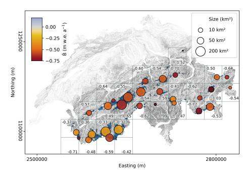
Figure 7. Area-weighted geodetic mass balance rates (colours and numbers) for  $30 \text{ km} \times 30 \text{ km}$  tiles (grey squares). The location of each circle is the average glacier centroid weighted by area in the tile, and their sizes indicate the glacier area in ca. 1931.
