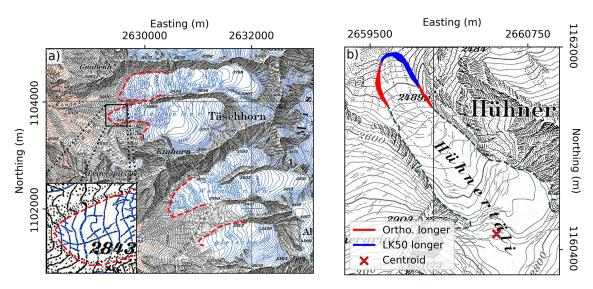
**Figure 5.** (a) Glacier outlines drawn from orthoimages generated in this study (dashed red), superimposed on a sheet of the LK50 map series. (b) Comparison between glacier outlines derived by digitising the LK50 map series and orthoimages. Red shading indicates that the outline drawn from the orthoimage is farther away from the centroid than the outlines derived from the LK50 map series. Blue shading indicates that they are closer.
