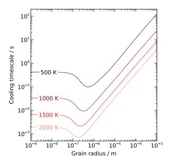
**Figure 9.** Cooling time-scales for graphite grains as functions of grain radius and temperature (Section 4.2.5). These are much faster than dynamical time-scales, so our assumption that escaping grains 'instantly' cool as their distance increases is valid.
