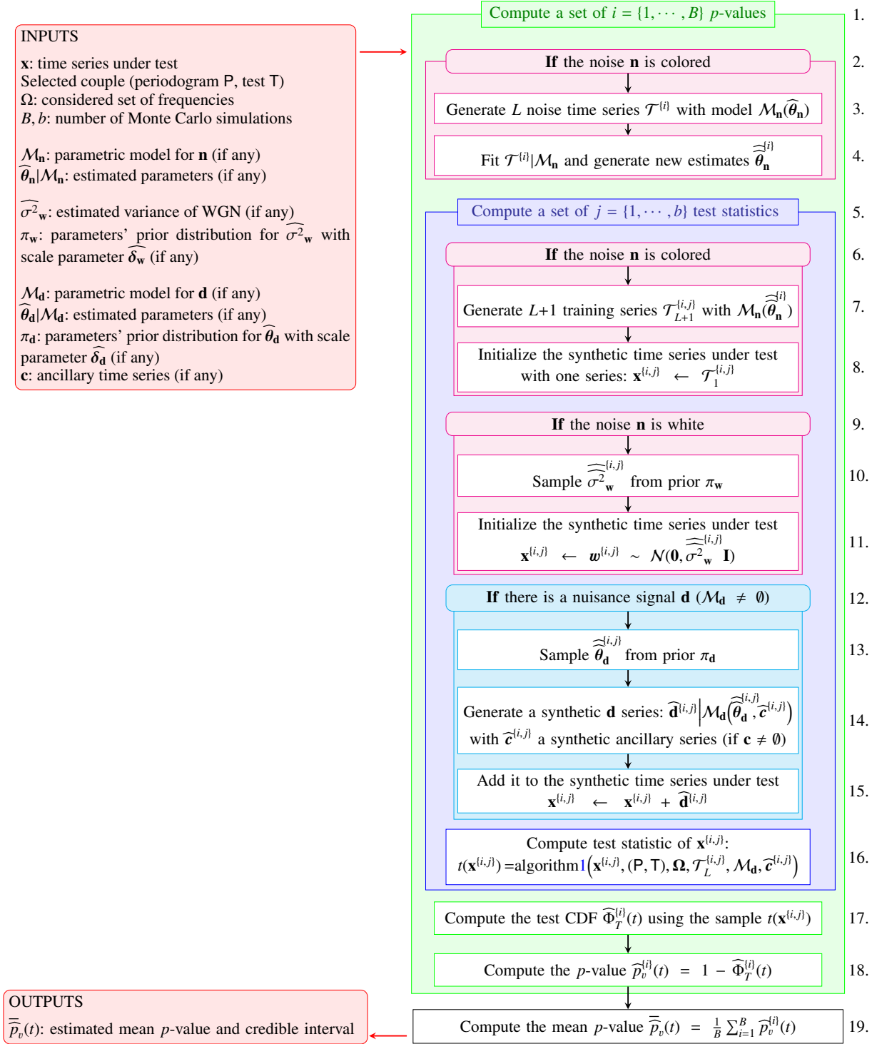
Fig. 2. Part of the 3SD procedure that estimates the p -value of algorithm 1 (algorithm 2).
