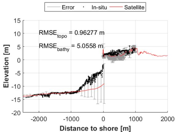
Figure 5. Comparison of in situ (black) and satellite-derived data (red) on a longshore median transect. The alongshore error between in-situ measurements and satellite estimate is represented as error bars (gray)
