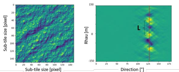
Figure 3. Raw offshore sub-tile from 03/2020 Pleiades imagery (2 m resolution pixel) (left) and its associated sinogram calculated with Radon Transform (right). The signal picked to estimate the waves parameters along the forced direction is in red, and the wavelength  $L$  corresponds to the distance between two intensity peaks.
