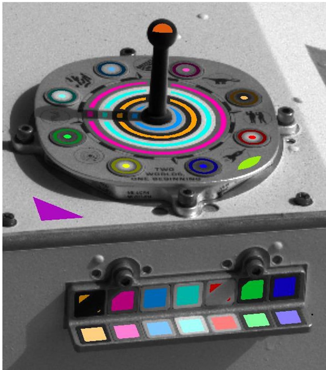
Figure 4. Example of regions of interest (ROI) selections over an image of the cal-targets taken by the left eye of Mastcam-Z in the L1 filter (800 nm) on sol 69 at 48 mm focal length (Image-ID: ZL1_0069_0673052731_973IOF_N0032208ZCAM03014_048085A03, seq. ZCAM03014). All 41 ROI are visible in colors, including those under the gnomon's shadow on the grayscale rings. The two ROI's partially selected in the secondary target were edited to exclude the shadows due to the bolts of the support.
