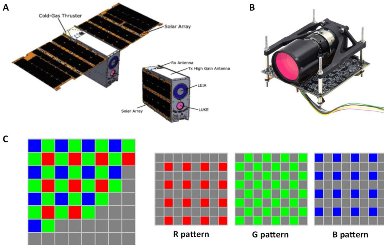
**Figure 1.** (a) A 3D model of LICIACube with the solar array deployed and closed. Labels mark some of the main components of the spacecraft and the position of two payloads, LEIA and LUKE, on board the spacecraft; adapted from Dotto et al. (2021). (b) Picture of the LUKE Gecko Imager for cubesat from SCS Space ([www.scs-space.com](http://www.scs-space.com)). (c) LUKE RGB Bayer pattern filter scheme and scheme of single color patterns.
