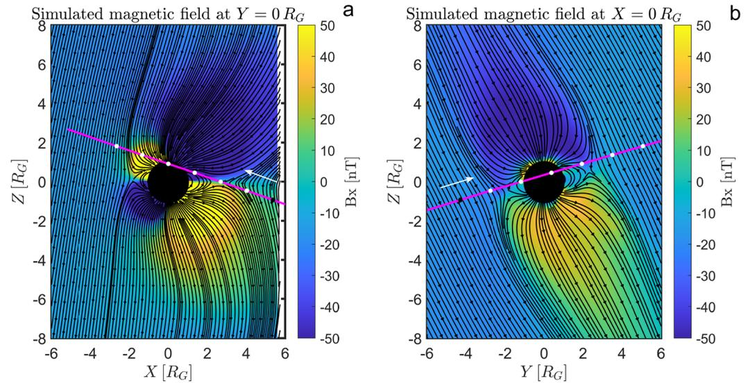
**Figure 1.** Simulated magnetic field  $B_x$  (Ganymede centered Phi-Omega) component at the  $Y = 0 R_G$  (panel a) and  $X = 0 R_G$  (panel b). Field lines (shown in black) are computed based on the magnetic field components contained in each of these planes. Juno's trajectory projections are shown by the magenta solid lines and the six dots show its location between 16:40 UT (black dot) and 17:10 UT, separated by 5 min intervals. The white arrows indicate the direction of increasing time.
