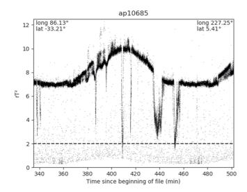
Figure 1.  $rT^2$  against time for a ~15 m window from orbital phase ap10. Series of several low  $rT^2$  returns are typical signatures of atmospheric structures while noise returns are sporadic decreases. Dashed line represents detection criteria used in Neumann et al. (2003). Some signatures appear as completely above this limit and may have been missed.
