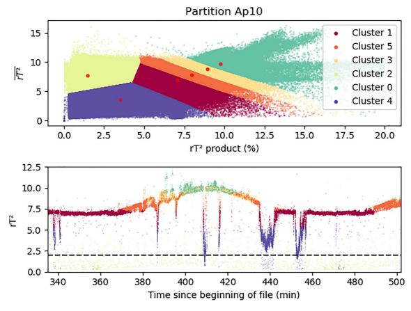
Figure 3. Example of clustering structure for ap10 orbital phase (a) and associated cluster distribution in the same  $rT^2$  against time portion than Figure 1b. Cluster 4 gathers cloud returns (bottom of troughs), cluster 2 is made of noise returns (isolated points). Clusters 0, 3, and 5 are surface returns (different parts of the continuum). Cluster 1 is a limit between continuum and troughs and ensure that no surface returns are taken in our cloud cluster.
