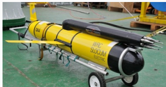
Microrider mounted on Slocum glider
