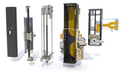
Fig. 2. From left to right, the drill box cover; the carrousel with three extension rods, plus a spare drill tool; the drill mandrel with its vertical traveling stage, depicted holding the main drill tool; the drill box with associated electronics (the CLUPI instrument can be seen on the lower left); and the drill attachment mechanism. Credits. ESA/Mlabspace.
