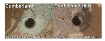
Fig. 5. Two examples of images of drill holes performed by NASA's Curiosity Rover respectively on Yellowknife Bay (Cumberland location, left image) and Confidence Hills (right image) in Gale Crater on Mars. The diameter of the holes is 1.6 cm. Images have been taken by the rover's Mars Hand Lens Imager (MAHLI) camera. From <a href="https://photojournal.jpl.nasa.gov/catalog/PIA21254">https://photojournal.jpl.nasa.gov/catalog/PIA21254</a>. Credits NASA/JPL-Caltech/MSSS/UA.
