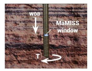
Fig. 3. Cross-section view of drilling into a sedimentary rock. The position of the Ma\_MISS window is  $\sim 22$  cm above the drill tip. The weight on bit (WOB) and torque (T) are among the most interesting parameters collected in the drill telemetry, providing information on the mechanical properties of rock layers. Modified from <u>https://bit.lv/</u>3bxe0M9 and Frigeri et al., (2021).
