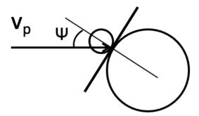
Fig. D.1: Schematic of the collision between a proton of initial velocity  $\mathbf{v}_p$  with a gas particle. The collision angle  $\psi$  is between the normal to the surfaces of the spheres at the point of contact and the proton velocity.
