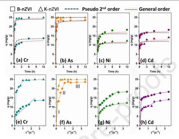
**Fig.5** (a-d) effect of interaction time, reaction kinetics modeling and (e-h) intra-particle diffusion (IPD) modeling of B-nZVI and K-nZVI for mono-ionic contaminant system [ $C_0$ = 20 mg/L, V= 25 mL, m= 20 mg, 200 RPM and 25°C,]
