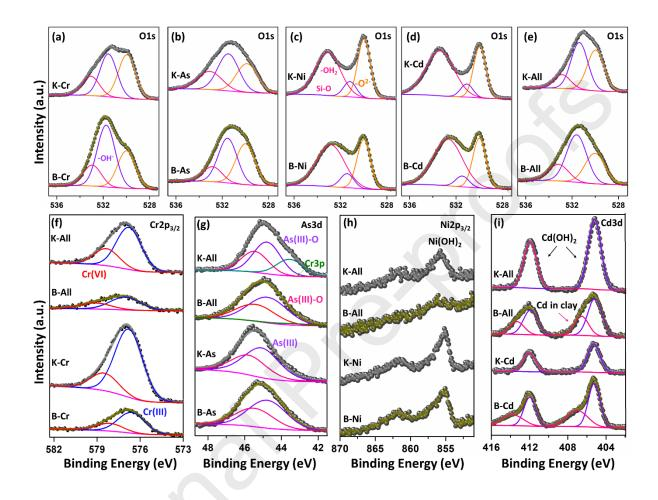
**Fig. 4** XPS data for different composites and reaction precipitates showing fitted (a-e) O1s spectra for reaction residues before and after sorption experiments for B-nZVI and K-nZVI, respectively, and spectral fits for (f)  $Cr2p_{3/2}$ , (g) As3d, (h) Ni $2p_{3/2}$ , and (i) Cd3d regions.
