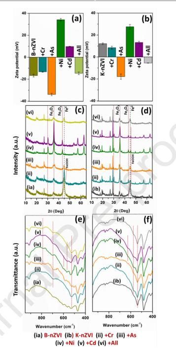
**Fig. 3** (a, b) zeta potential, (c, d) pXRD and (e—f) FTIR spectra obtained for different reaction precipitates after sorption experiments using B-nZVI and K-nZVI respectively [(ia) B-nZVI, (ib) K—nZVI, (ii) Cr, (iii) As, (iv) Ni, (v) Cd, and (vi) Cr-As-Ni-Cd].
