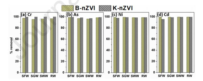
**Fig.8** removal of various metallic species from different aqueous matrices [m= 20 mg, V= 20 mL,  $C_0= 10 \text{ mg/L}$ , T= 25<sup>o</sup>C, RPM= 200, t= 12h]
