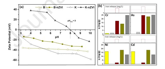
**Fig.2** (a) Zeta potential at varying pH for clays and synthesized nanocomposites and (b) Sorption capacity of raw constituents of nanocomposites i.e., Bentonite, Kaolinite and nZVI
