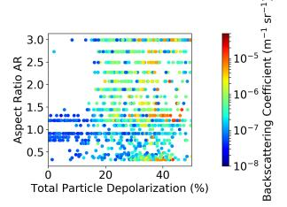
**Figure A7.** Scatterplot of the total particle depolarization vs. the aspect ratio, color coded in terms of the backscatter coefficient.
