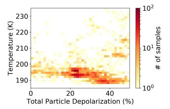
**Figure 2.** A 2D histogram of total particle depolarization data vs. temperature for altitudes above 11 km. Data were acquired throughout the campaign by the MAS backscattersonde. The color codes indicate the number of observations in the 2D bin, representing 2308 data points.
