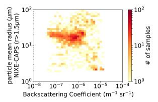
**Figure 8.** A 2D histogram of particle backscattering coefficient observations  $\beta$  from the backscattersonde MAS and particle mean radius  $R_{\text{mean}}$ . Data were acquired throughout the campaign by the MAS backscattersonde. The color codes represent the number of observations in the 2D bin.
