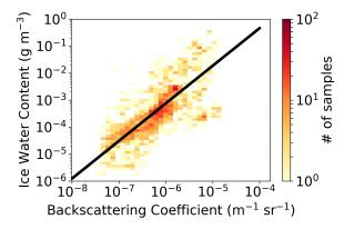
**Figure 11.** A 2D histogram of particle backscattering coefficient observations from the backscattersonde MAS and ice water content (IWC). The black line represents the fit IWC =  $1.78 \times 10^5 \cdot \beta^{1.39}$ . The color codes represent the number of observations in the 2D bin.
