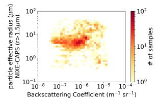
**Figure 9.** A 2D histogram of particle backscattering coefficient observations  $\beta$  from the backscattersonde MAS and particle effective radius  $R_{\rm eff}$ . Data were acquired throughout the campaign by the MAS backscattersonde. The color codes represent the number of observations in the 2D bin.
