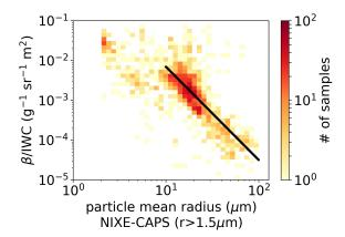
**Figure 17.** A 2D histogram of the ratio of the backscattering coefficient in relation to IWC versus particle mean radius. The black line shows a regression computed for  $R_{\rm mean}$  from 10 to 100 µm. The fit is  $\frac{\beta}{\rm IWC} = 1.53 \cdot R_{\rm mean}^{-2.34}$ , with an R-squared value of 0.54. The color codes represent the number of observations in the 2D bin.
