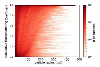
**Figure 16.** A 2D histogram of cumulative distributions of particle backscattering coefficient computation. The histogram shows the buildup of the particle backscattering coefficient with respect to the particle radius for all the PSDs under study. For the present graph, Mie scattering computation has been used.
