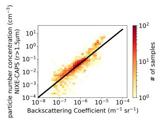
**Figure 7.** A 2D histogram of particle backscattering coefficient observations  $\beta$  from the backscattersonde MAS and particle number concentration N. The black lines represent the fit  $N = 3.96 \times 10^6 \cdot \beta^{1.32}$ . Data were acquired throughout the campaign by the MAS backscattersonde. The color codes represent the number of observations in the 2D bin.
