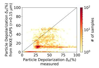
**Figure 6.** 2D histograms of occurrence of the measured and calculated particle depolarization. Data were acquired throughout the campaign by the MAS backscattersonde. The color codes the number of observations in the 2D bin.
