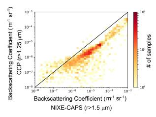
**Figure A6.** A 2D histogram of the backscattering coefficient computed from PSD from NIXE-CAPS (x axis) and CCP (y axis). For NIXE-CAPS, only particles with a lower size limit of 1.5  $\mu$ m have been considered. The computation was performed with Mie scattering codes.
