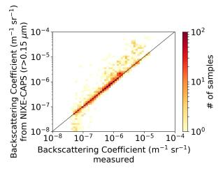
**Figure 5.** 2D histograms of occurrence of the measured and calculated backscattering coefficients. Data were acquired throughout the campaign by the MAS backscattersonde. The color codes the number of observations in the 2D bin.
