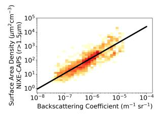
**Figure 10.** A 2D histogram of particle backscattering coefficient observations  $\beta$  from the backscattersonde MAS and particle surface area density (SAD). The black line represents the fit SAD =  $7.07 \times 10^8 \cdot \beta^{1.11}$ . The color codes represent the number of observations in the 2D bin.
