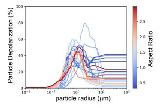
**Figure A2.** Particle depolarization vs. particle radius for various choices of the aspect ratio. The black zero-depolarization line refers to Mie computations (AR = 1). For particle radii below 14  $\mu$ m, the computations were performed with the GRASP package. Beyond 14  $\mu$ m, for every given AR, the depolarization of the particles was set at its constant, asymptotic value, computed as its mean over the particle radius dimensional region from 5 to 14  $\mu$ m (60–180 size parameters).
