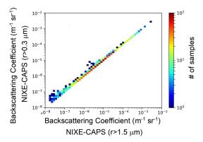
**Figure A3.** A 2D histogram of the backscattering coefficient computed with PSD with lower size limits of  $0.3 \, \mu m$  (y axis) and  $1.5 \, \mu m$  (x axis). A spherical ice approximation has been used in the computation.
