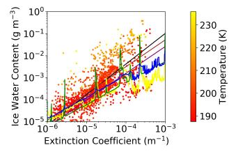
**Figure 18.** Scatterplot of measured IWC vs. estimated extinction  $\sigma = 30\beta$ . The solid lines represent regressions from (i) the present work, black; (ii) Heymsfield et al. (2005), purple; (iii) Avery et al. (2012), brown; Heymsfield et al. (2014), yellow and green; Thornberry et al. (2017), blue. Experimental points are color coded in terms of the temperature of the observation.
