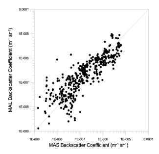
**Figure 4.** A 2D histogram of particle backscatter coefficient observations from the backscattersonde MAS and the particle backscattering coefficient data from the two MALs, pointing upwards and downwards, at 500 m from the aircraft. The average of the two lidar backscattering coefficients has been used for the comparison. The data have been averaged over 60 s. In the graph are the 500 data points acquired while crossing some of the thickest clouds observed during the campaign.
