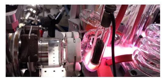
Figure A1-2: Configuration with the MS collecting head close to the plasma (~5 cm).
