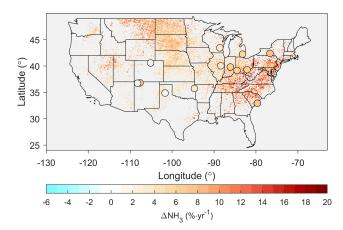
**Figure 6.** Trend analysis for IASI NH<sub>3</sub> (2008–2018) and AMoN NH<sub>3</sub> measurements in the contiguous US. The gray color indicates no statistically significant change ( $\alpha = 0.05$ ).
