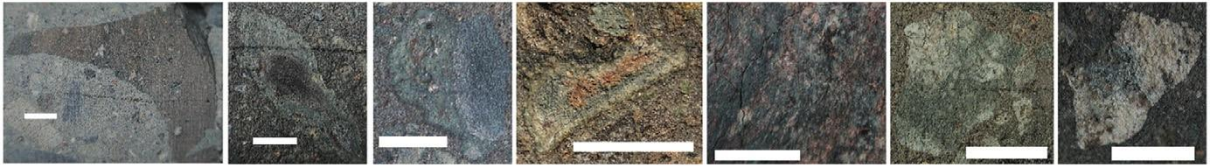
Brown w. lithic fragments 49.580 m depth Green and brown 14.515 m depth Green w. clast (right) 15.805 m depth Green w. lithic core (red) 8.055 m depth Dark green 26.330 m depth Green and white 32.105 m depth White (w. green) 14.550 m depth
