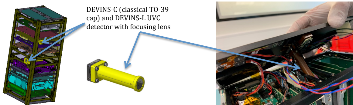
Figure 10. Illustrative view of the DEVINS detectors positions on the nanosatellite INSPIRE-SAT 7 and photo of DEVINS-L integration in the nanosatellite (Credits: INSPIRE-SAT 7).
