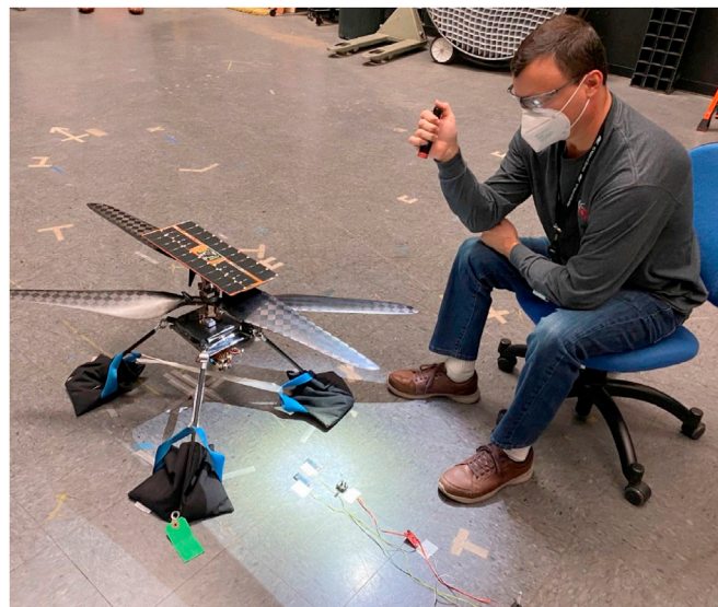
Fig. A4. Demonstration helicopter “Terry” secured to the laboratory floor by weighted bags. The investigator is holding a flashlight that illuminates two photodiode sensors underneath the rotor blades so that readings from pressure and acoustic sensors could be synchronized with blade passage via the shadow signals. The investigator is masked per Aerovironment policy at this stage of the Covid pandemic (September 2021).
