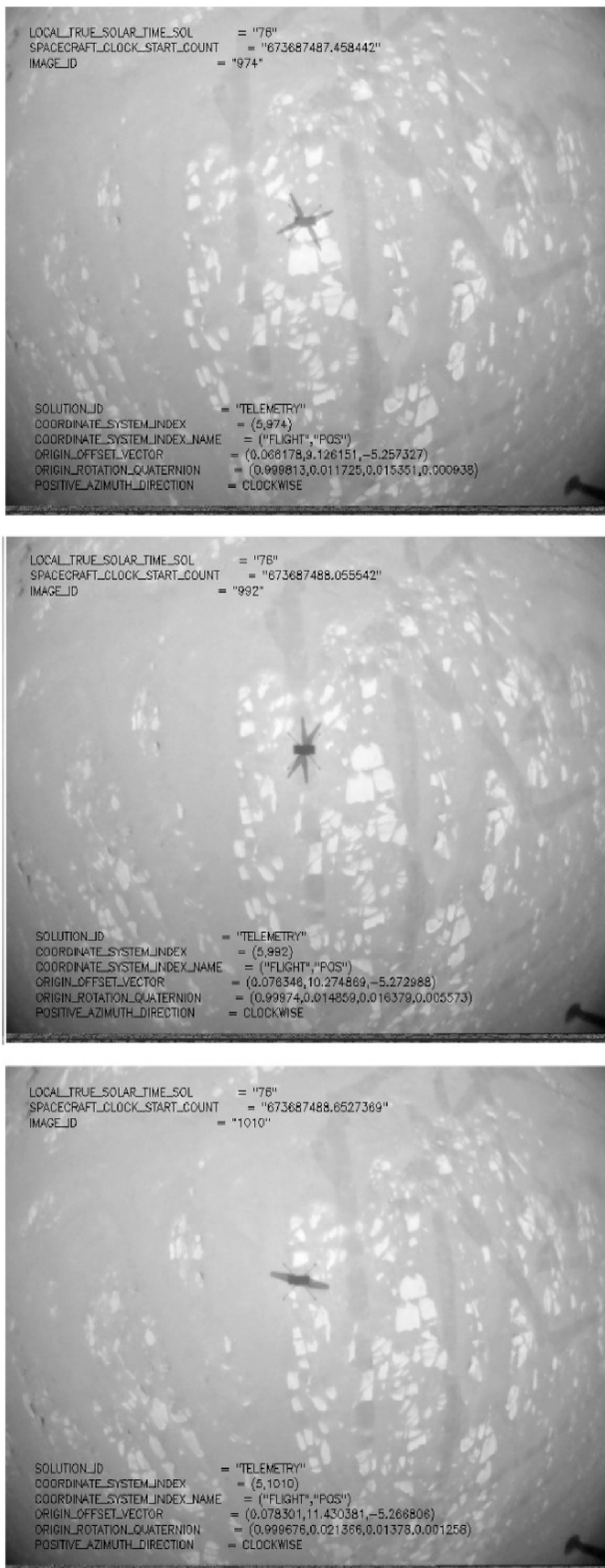
Fig. 15. Navigation Camera frames from flight 5, annotated with metadata from the image headers. The image numbers increment by 28, as only a subset of images were sent to Earth, and are separated by about 0.6 s. The helicopter is flying towards the left, so the scene (grey sand, with slightly darker rover tracks, and slabs of bright rock) moves towards the right, whereas the shadow of the helicopter remains fixed in the center. The shadows of the rotor blades rotate between frames: the stroboscopic snapshots occasionally show the blade crossing (bottom panel).
