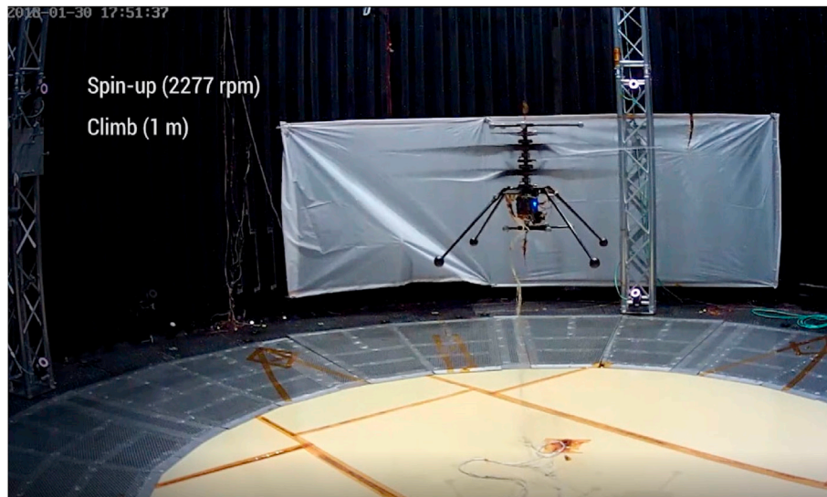
Fig. A2. Hover test in chamber at Mars pressure.
