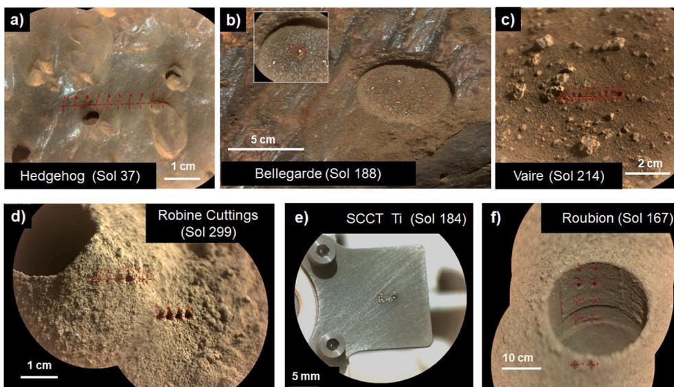
**Fig. 3.** Image of several examples for a) Bulk targets; b) Abraded patch; c) Regolith; d) Drill Tailings; e) Titanium SCCT, and f) Sample Collection Hole. The black labels represent the target name, and the red crosses the LIBS sampling position. Links to the images: Annex I on the Supplementary material document. (For interpretation of the references to colour in this figure legend, the reader is referred to the web version of this article.)
