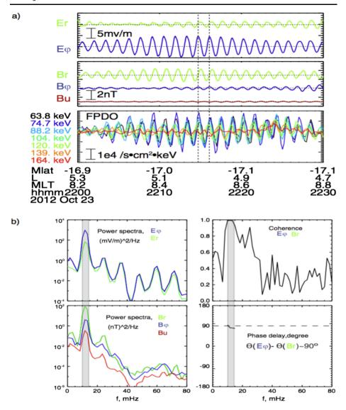
**Fig. 6** (Adapted from Dai et al. 2013) Fundamental mode standing poloidal wave with electric and magnetic fields in drift resonance with 63–164 keV ring current ions (Panel a). The results of a spectral and coherence analysis between the wave components are shown in Panel **b**
