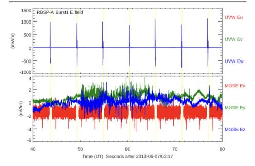
Fig. 28 Forty seconds of burst 1 electric field data showing the effects of spikes caused by shadowing of the  $V_5$  boom by the spin plane wires. The shadowing, with times indicated by the yellow lines, is observed in (a) the  $E_w$  UVW component, which is derived from the potential difference  $V_5 - V_6$ . (b) The electric field rotated to MGSE coordinates after removal of the spikes.  $E_x$  MGSE is equivalent to  $E_w$  UVW
