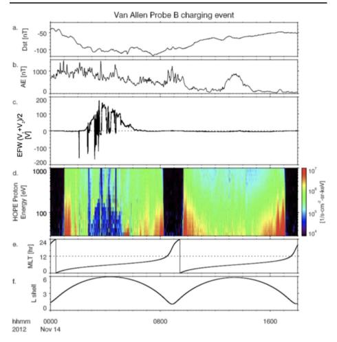
**Fig. 26** Van Allen Probe B charging during the 2012-11-14 geomagnetic storm. Panels  $(\mathbf{a}, \mathbf{b})$  show DST and AE indices. Panel  $(\mathbf{c})$  plots the negative spacecraft potential  $-V_{sc}=(V_1+V_2)/2$ . Panel  $(\mathbf{e})$  shows the HOPE proton energy spectrum modified by the excessive spacecraft charging. Panels  $(\mathbf{f}, \mathbf{g})$  show the magnetic local time and L-shell of Van Allen Probe B
