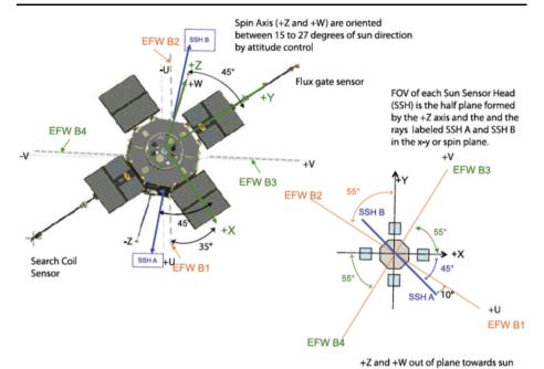
Fig. 23 (Adapted from Wygant et al. 2013) The orientation of the EFW spin plane boom sensors (u, v, w coordinates) on the Van Allen Probes spacecraft
