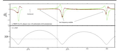
Fig. 29 An example of oscillations in the 32 Samples/sec spin plane electric field following an attitude adjustment maneuver on RBSPa near 15 UT on Jan 10th, 2013. E<sub>V</sub> MGSE is green and E<sub>Z</sub> MGSE is red
