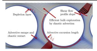
FIG. 3. Near-interface dynamics controlling the restart time in fully-chaotic, no-slip flow. Under fully-chaotic advection in the bulk, dynamics near no-slip interfaces represent the limiting factor for advection-induced exploration of the domain and set the restart time. This leads to restart times controlled by interface shear  $\gamma$ , which result from balancing advective and diffusive escape times near the interface.
