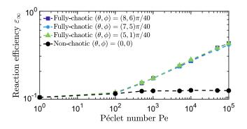
FIG. 2. Asymptotic reaction efficiency as a function of Péclet number for Stokes flow through a BCC, for Damköhler number  $10^2$  and four flow orientations, three yielding fully-chaotic (squares:  $\lambda_{\infty} \approx 7.53 \times 10^{-3}$ ; triangles:  $\approx 1.40 \times 10^{-1}$ ; asterisks:  $\approx 2.52 \times 10^{-1}$ ) and one nonchaotic flow (circles).
